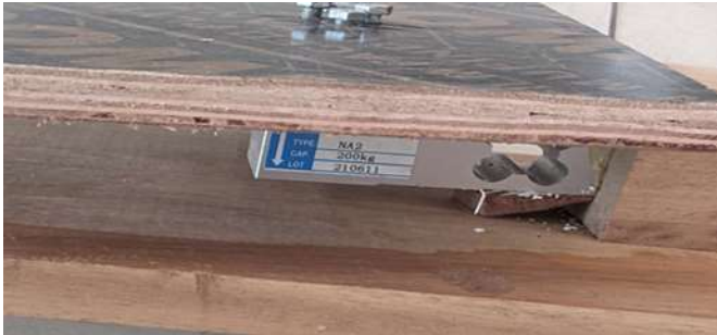
Figure 3-10 weight sensor supported under wooden structure
