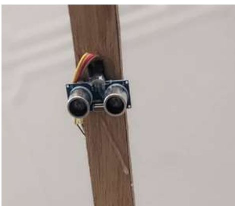
Figure 3-11 mounted ultrasonic sensor on wooden structure
