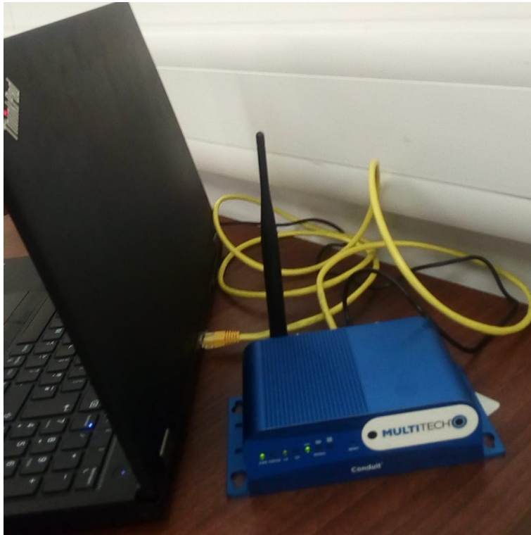
Figure 6.11: LoRaWAN gateway set up..
