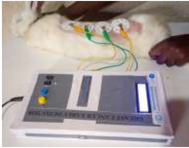
Figure 4.1: Breast cancer early detector under test on rabbit.
