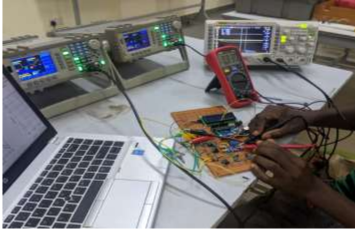
Figure 3.22: Testing phase detector on an oscilloscope.
