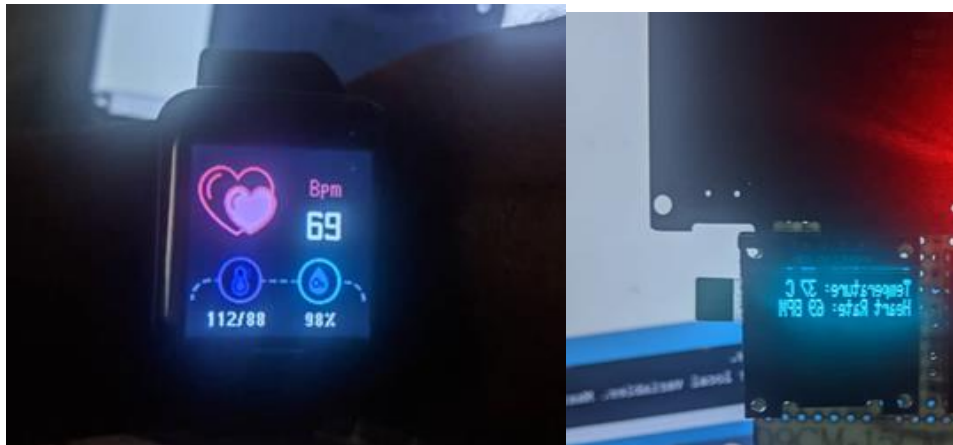
Figure 4.2: measurement of heartrate by using smart watch vs prototype
