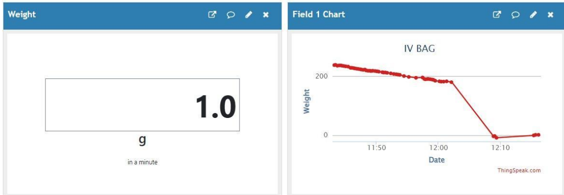
Figure 5. 6: the weight of the remaining intravenous are updated on the graph
