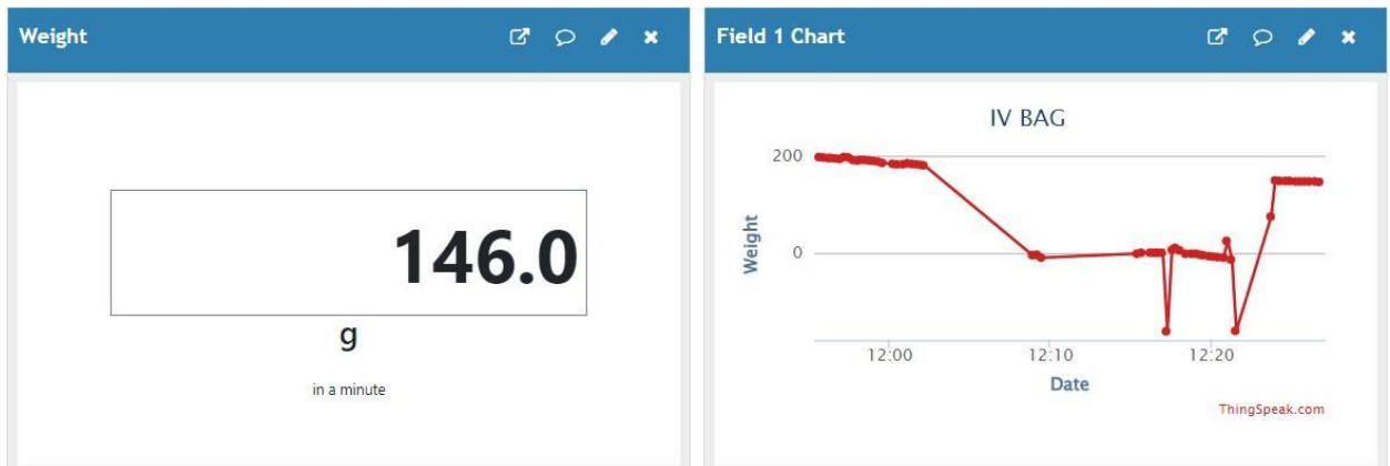
Figure 5. 4: the weight of the IV bag is seen also on ThingSpeak
