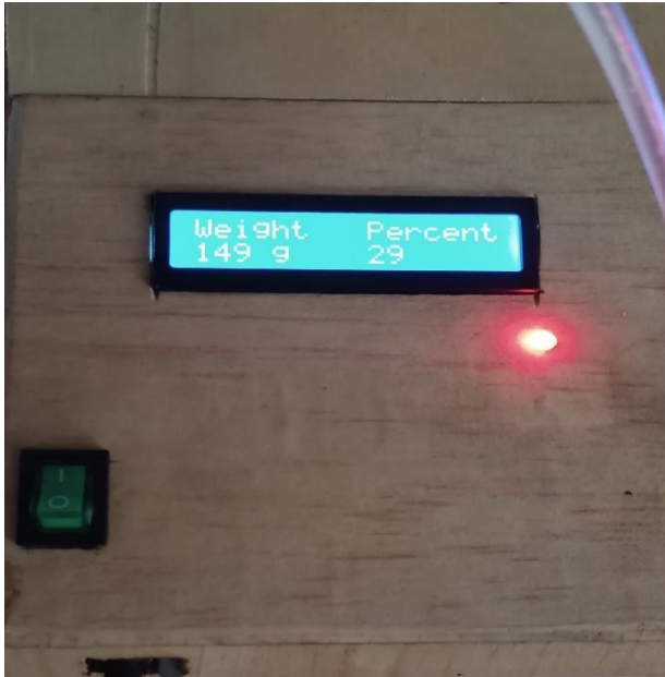
Figure 5. 3: the weight of IV bag is displayed on LCD display
