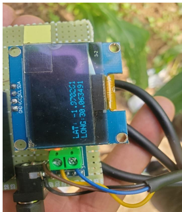
Figure 6: GPS coordinates being captured by the IoT device
