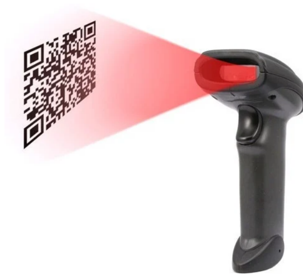
Figure 2.2: Bar code reader [10]
