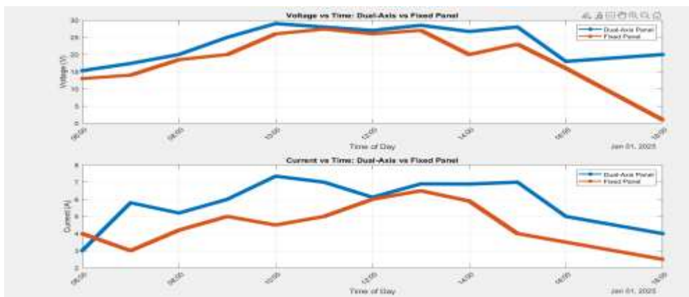
Figure 4.9: Output voltage and current vs time for both fixed panel and moving panel
