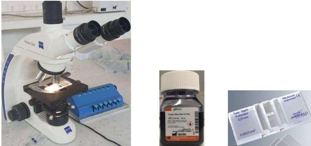
Figure 5: Zeiss Microscope (left side), Trypan blue (in the middle) and Hemocytometer (Improved new Bauer on the right side)
