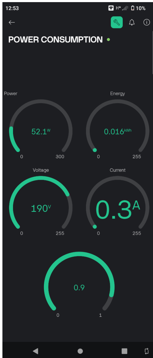
Figure 4. 9: Blynk widget monitoring of energy usage on smart phone
