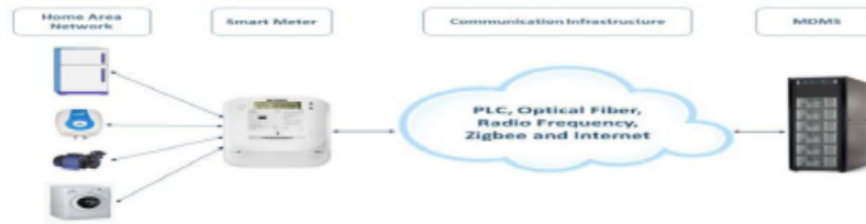
Figure 2.18 Graphical relationship of the AMI system [56]
