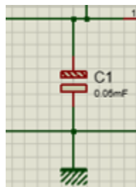
Figure 4.6 Filtering capacitor design
