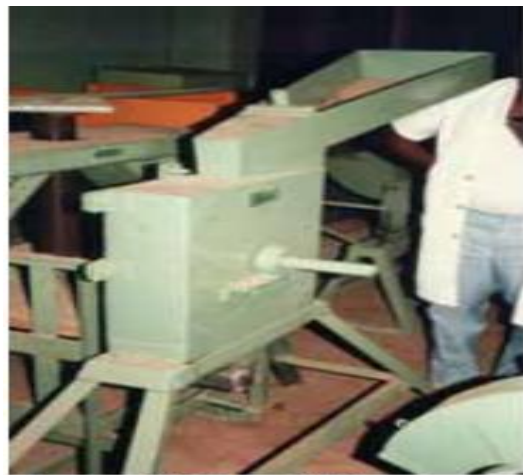
Figure 4-6: Pounding by with mortar and pestle Figure 4-7: Pounding by grain mill driven by motor
