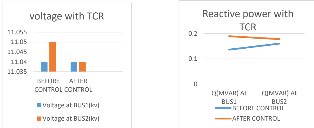
(a)Voltage before and after TCR connected (b)Reactive power before and after controller
