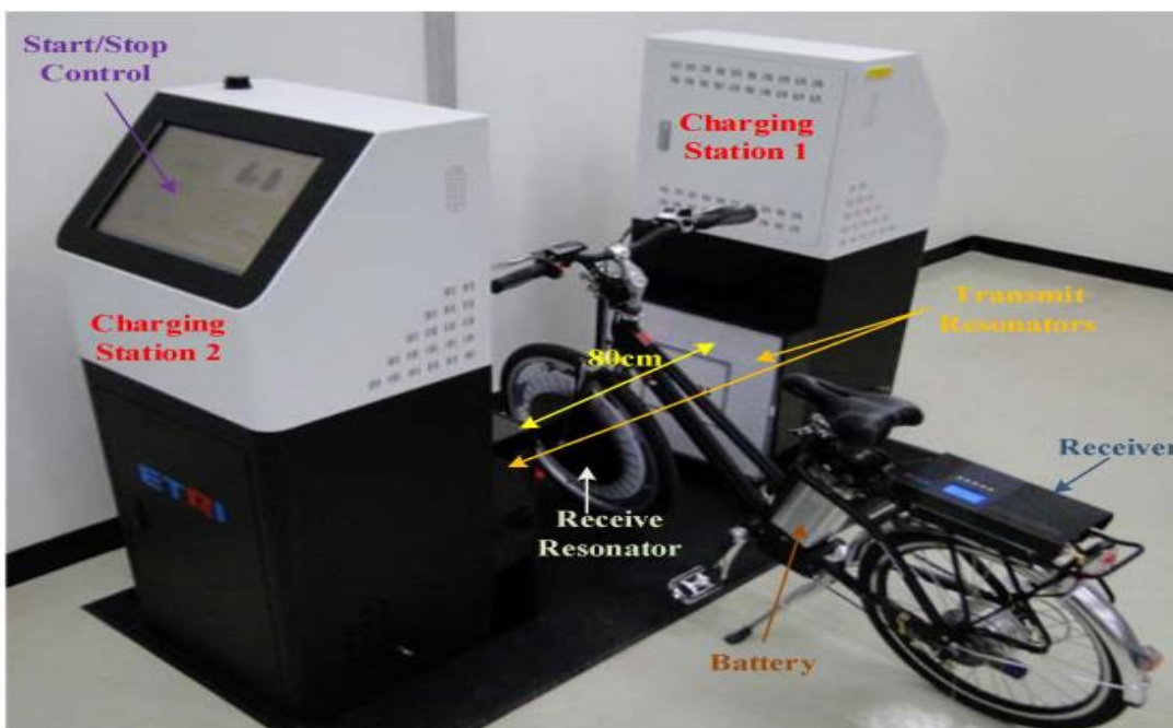
Figure5. 7 constructed Electrical wireless charging system for E-bike [32]
