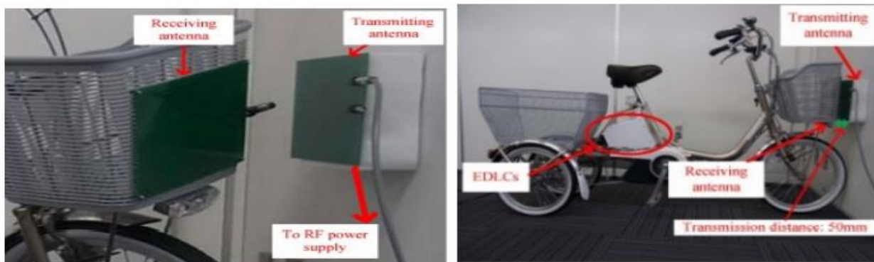
Figure3. 7:methods of wireless charging of the electric[22]
