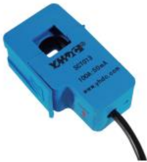
Figure 3. 7: Current sensor SCT013[22].
