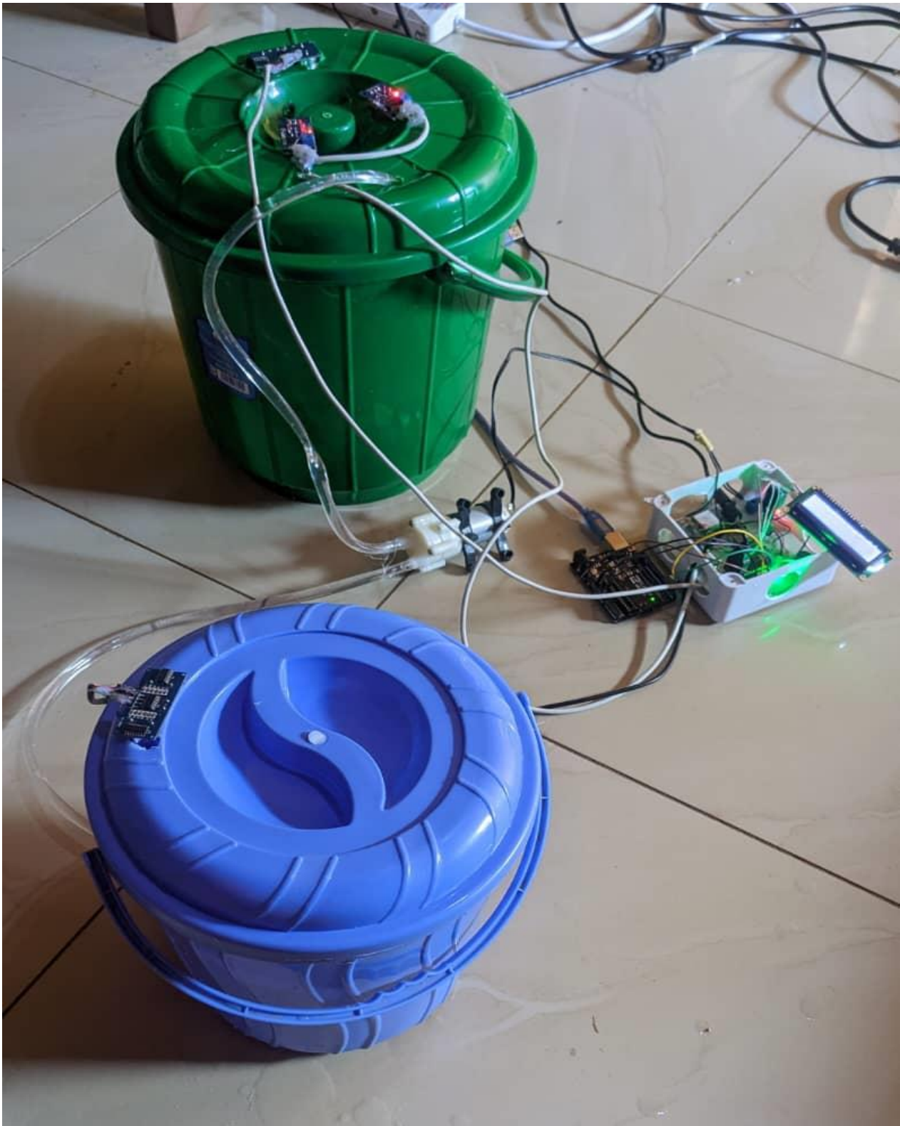
Figure 5. 3: Complete experimental setup of IoT based septic tank monitoring system
