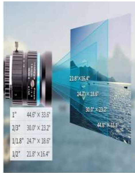
Figure 3-11: Field of view of HQ camera
