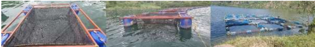
Figure 3: Floating system made up of metallic frames and plastic drums (Source: Author, 2022).
