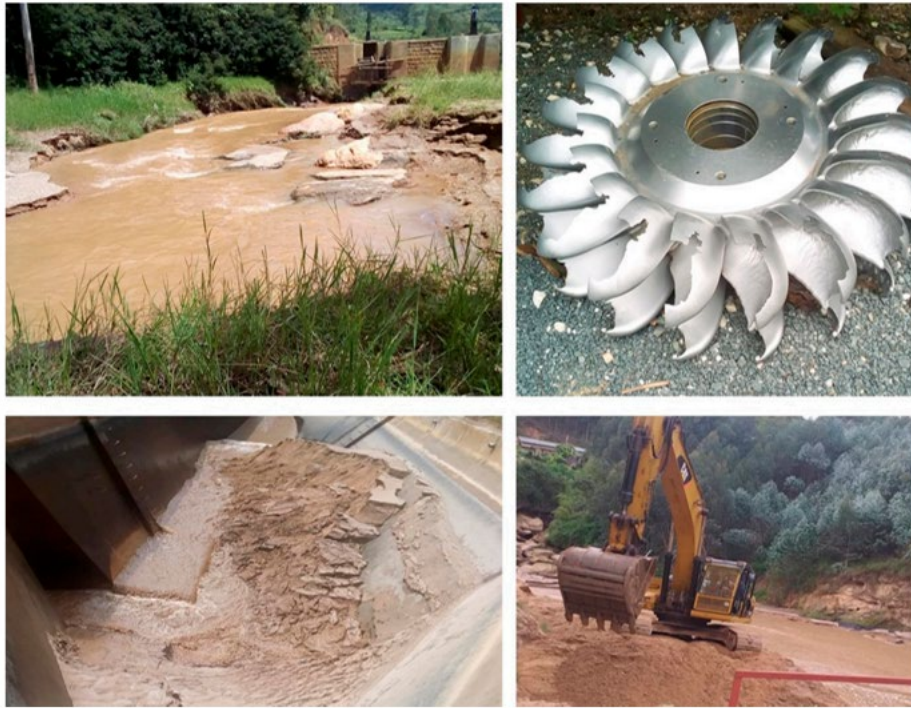
Figure 8. Field observation on soil erosion, sediments, and turbine wear. Clockwise from upper left: an upstream catchment filled with sediments and soil erosion during one rainy season, turbine runner wear due to waterborne sediment after 1.5 years in operation, heavy equipment removing sediments from another upstream catchment, and a sediment basin filled by sediments over three days during rainy season.
