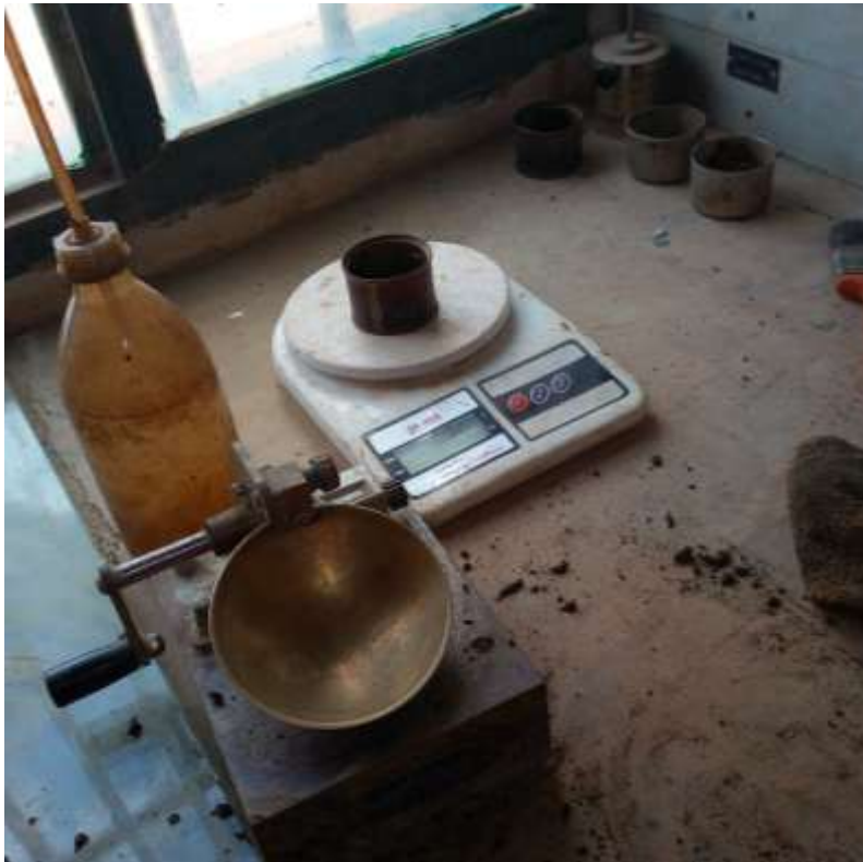
Figure 3- 7 Casagrande apparatus to perform liquid limit (LL)
