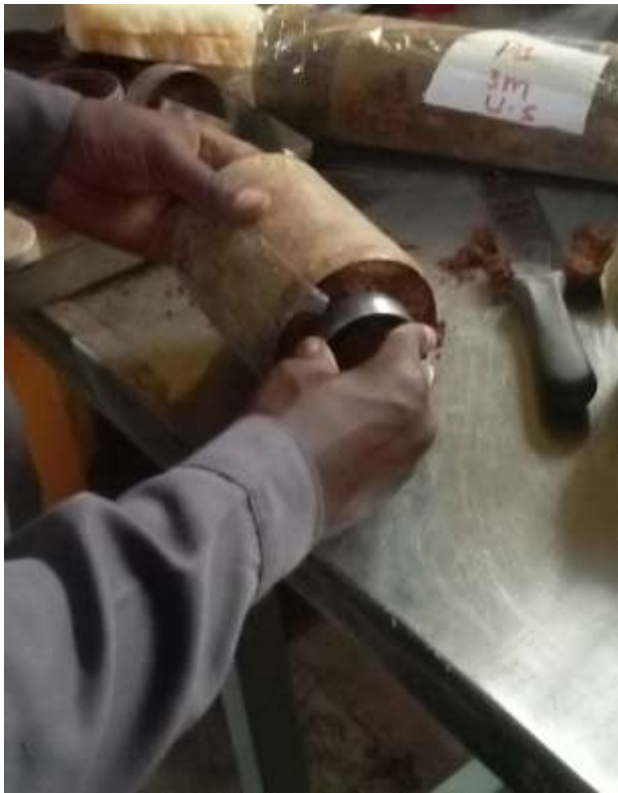
Figure 3- 4 Putting the sample in the sampler for direct shear and unit weight determination
