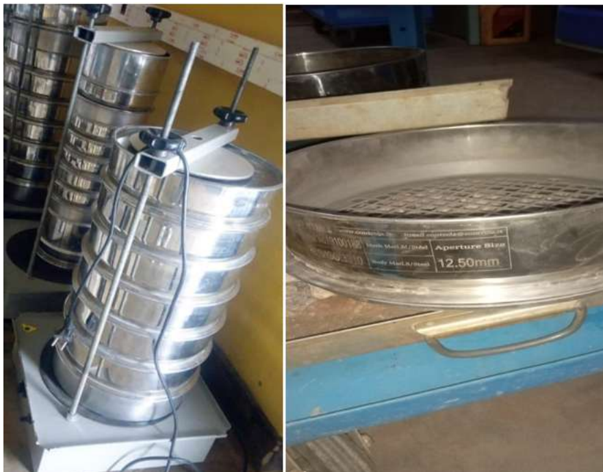
Figure 3- 3 Sieve shaker and sieve mesh used in grading analysis
