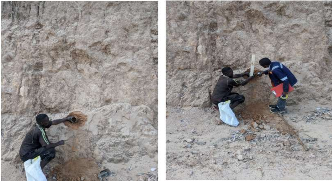
Figure 3- 1 Sampling an undisturbed sample slided portion of a road Huye-Nyamagabe road
