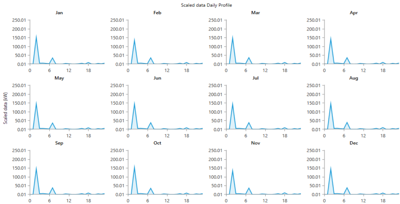
Figure4.20 Time series Analysis of yearly hour of each month against load power in Kw
