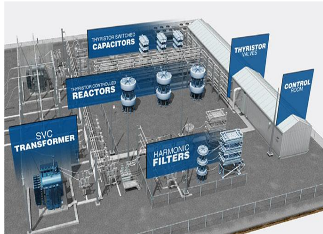
Figure 2: SVC Power Delivery Projects Grid Solutions
