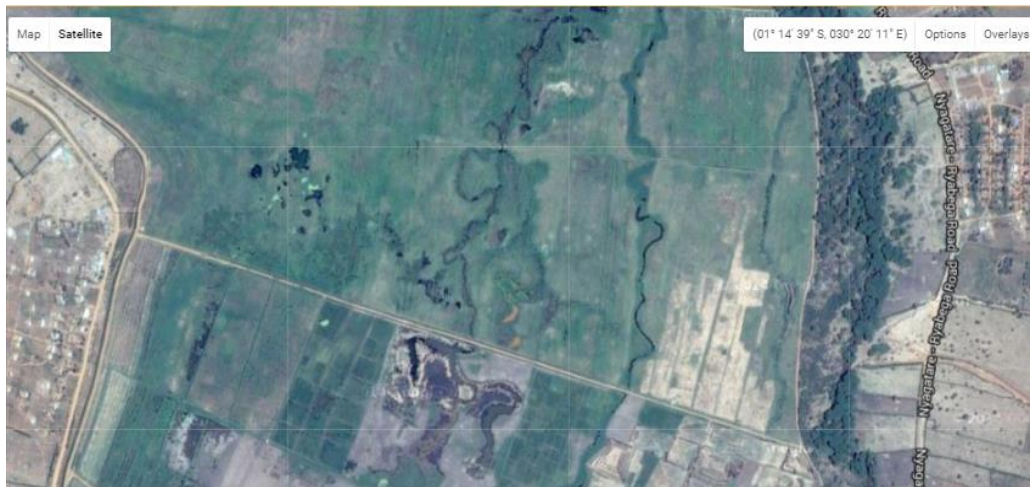
FIGURE 10: SATELLITE IMAGERY SHOWING STAGNATE WATER DUE LEVELING ISSUES, 2016
