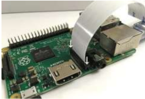
Figure 13: Pi camera connected to Raspberry Pi
