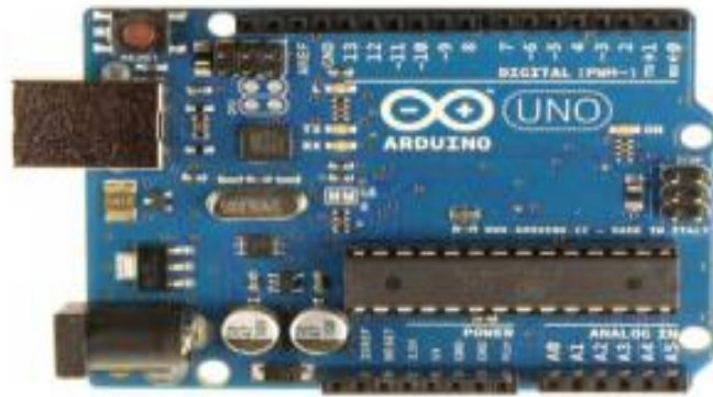
Figure 3.2 Arduino uno used in the circuit
