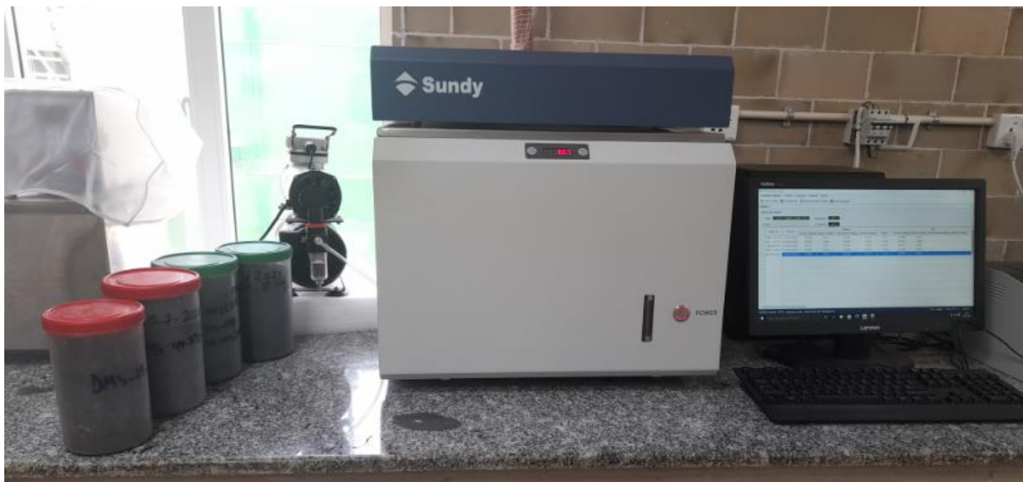
Photo 9: Proximate analysis by SD-TGA proximate analyzer
