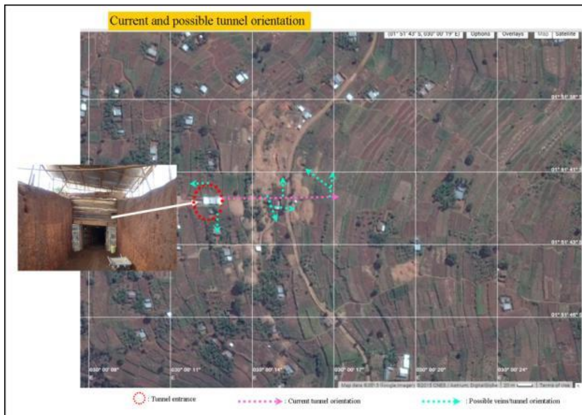
Figure 19: Current and possible tunnel orientation Source: field observation, 2016
