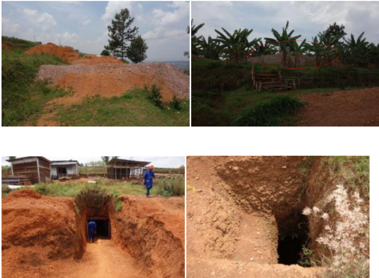
Figure 18: Tailings deposits in the croplands, operational tunnel and one of the scattered shafts Source: Field observation, 2016
