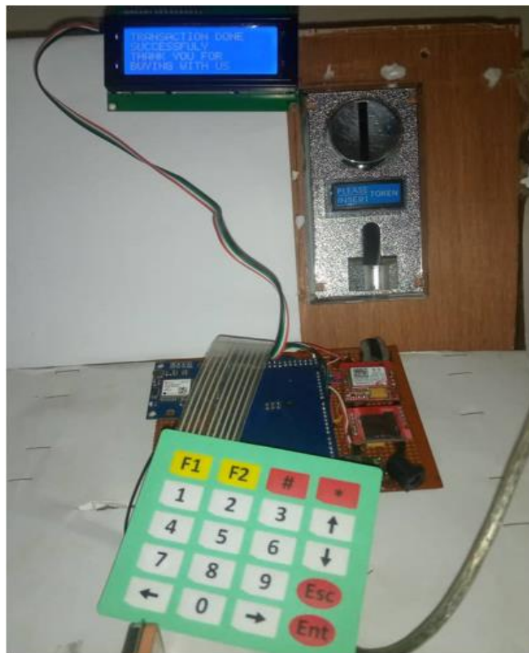
Figure 19: Fixing of vending machine components
