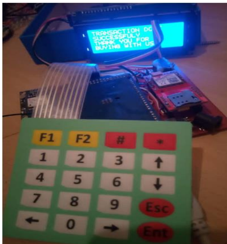
Figure 18: Interconnection of vending machine components
