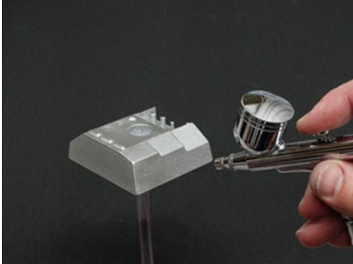
Figure 5.5: Spray painting process
