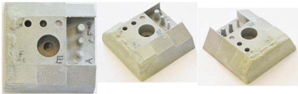
Figure 5.10: Effects of resorcinol and nitric acids on surfaces of Alumide® test pieces
