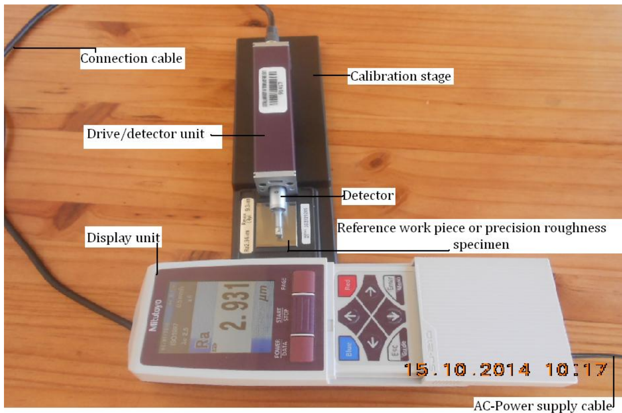
Figure 6.1: Main units of the surface roughness measurement tester SJ-210
