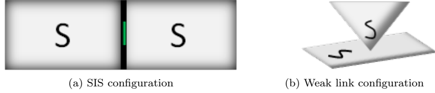
Figure 2.5: Josephson junction. S represents the superconductive component and I the insulator.
