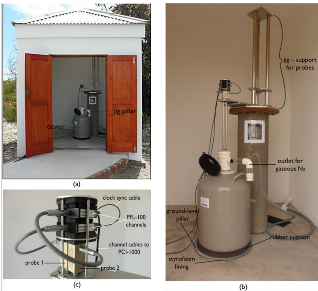
Figure 5.13: Depiction of the SQUID system in Hermanus (a) non-magnetic hut housing the SQUID (b) A view inside the hut showing the full installation of SQUID in the Dewar flask (c) a close-up view of the Programmable Feedback Loop (PFL) controllers [16].
