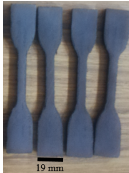
Figure 3.14: Prepared tensile test specimen
