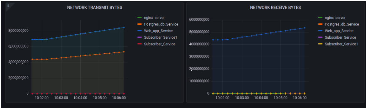
Figure 5. 19: Performance of the platform after scaling up with requests to 1000 network data transmissions.
