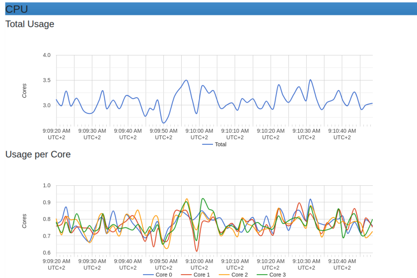
Figure 5. 14: CPU resources with 10,000 generated sensor requests.
